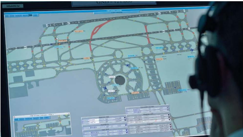
and ground control personnel with specific information about the location and speed of aircraft. Because it works at low altitudes and on the ground, ADS-B provides a significant advantage over traditional radar. It means that ADS-B can be used to monitor traffic on the taxiways and runways of an airport, thereby significantly improving safety on the airport surface.
