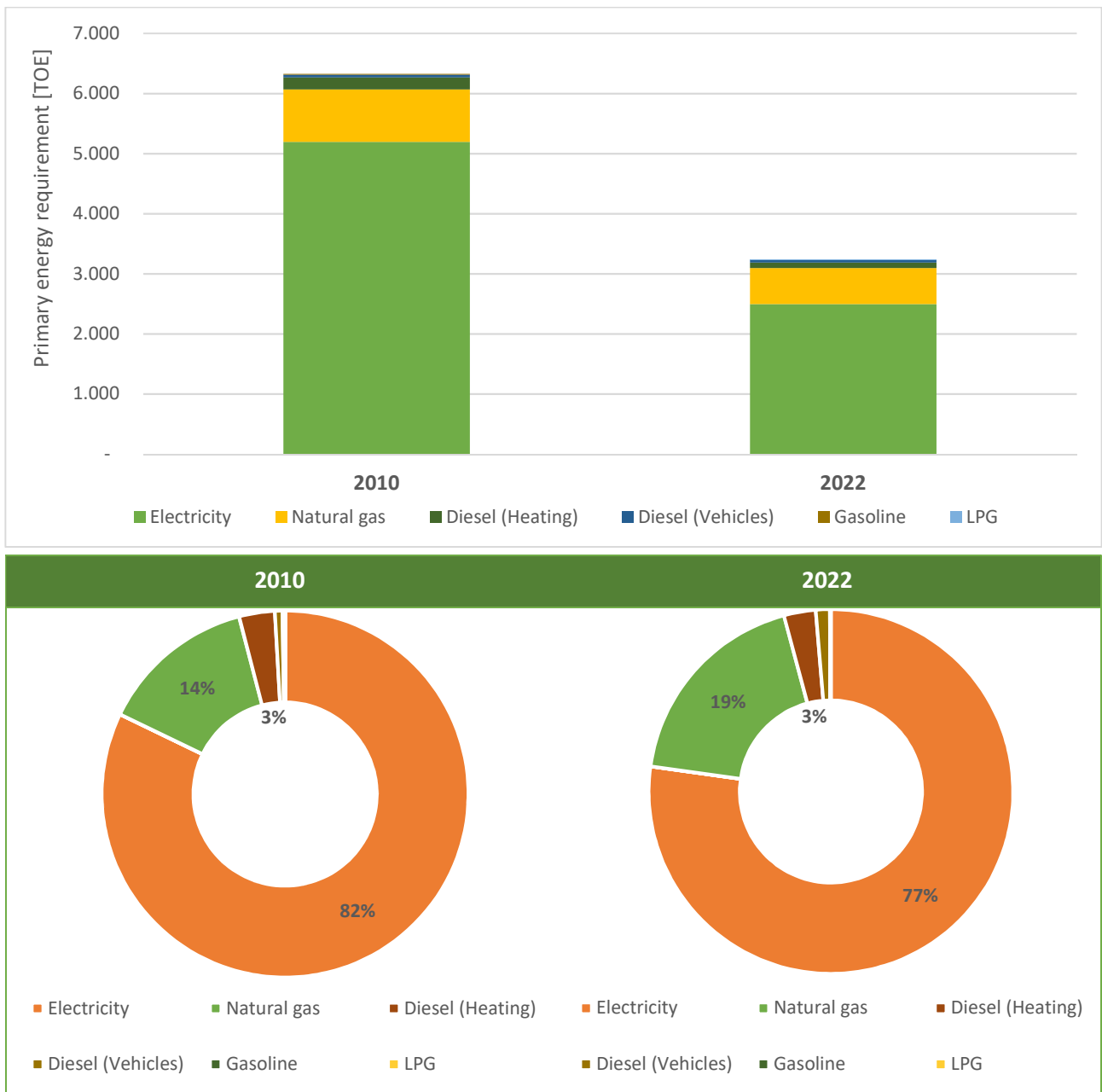
Figure 1 - Comparison of primary energy requirements by carrier years 2010 and 2022
